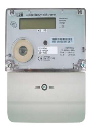
The electricity meter ZE114 series is a modern, fully programmable meter for monitoring the consumption of electric energy in low-demand areas. It is able to meet the monitoring requirements of active energy accuracy class A or B. Its structure is designed to connect to the network TN-C.
