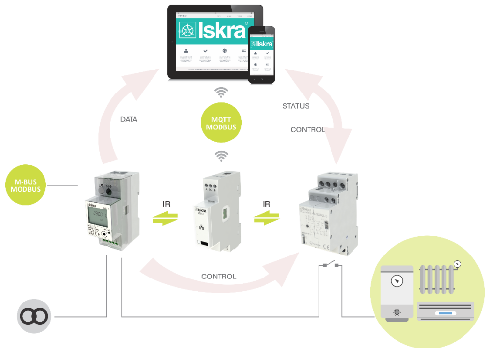
Figure 2: Connection diagram for SG. It is connected to an energy meter (on the left side of the SG) and to latching switch (on the right side of the SG) by IR communication. It is possible to read and control data with the computer or mobile phone.
