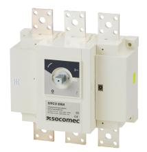
SIRCO are manually or remotely operated multipolar load break switches. They make and break under load conditions and provide safe isolation. SIRCO are designed for 415 VAC and DC low voltage electrical circuits.
